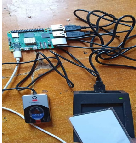
Figure 3: Connections of GT-521F52 fingerprint module, RFID reader and tag around Raspberry Pi 4 microcontroller.
