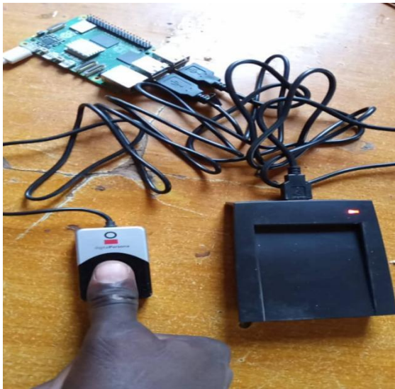
Figure 4: Testing the programmed Raspberry Pi 4 with the GT-521F52 fingerprint sensor module.
