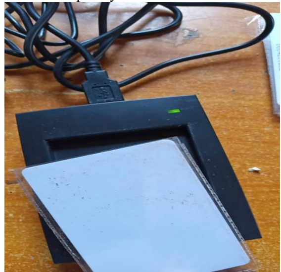
Figure 5: Testing the configured RFID card on the reader for RC4 authentication and functionality.
