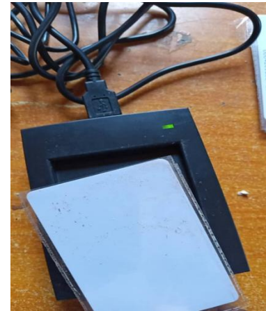
Figure 6: Testing the RFID card on the RFID reader for RC4 authentication.
