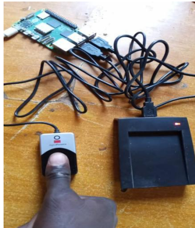
Figure 5: Testing the GT-521F52 module with Raspberry Pi 4 using a real fingerprint.
