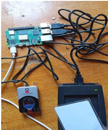
Figure 4: GT-521F52 fingerprint module, RFID reader and tag connected to Raspberry Pi.
